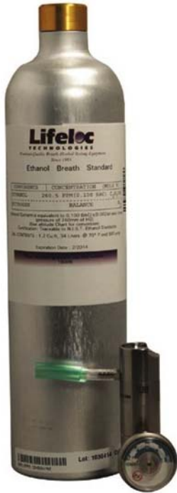
Figure 2: A common 34 Liter NIST traceable Dry Gas Cylinder and Regulator.
