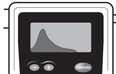
If the FC10 detects alcohol, the alcohol level is graphed and will be displayed before the result.
