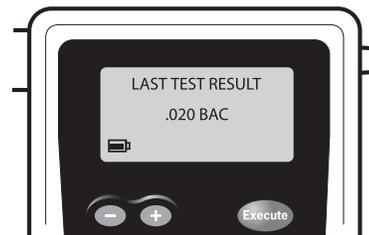
Press the **Function** button until "LAST TEST RESULT" is displayed. The results of the last test will be displayed.
